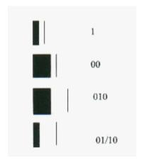
There are four possible combinations of wide and narrow bars and spaces. Ideally one would like these to represent binary data in order to simplify decoding.
